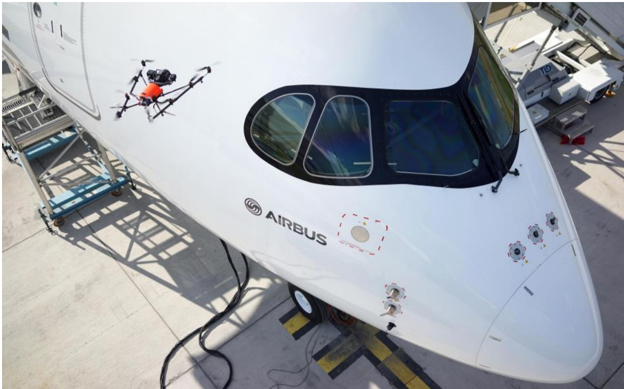
A350 XWB quality inspection by drone
