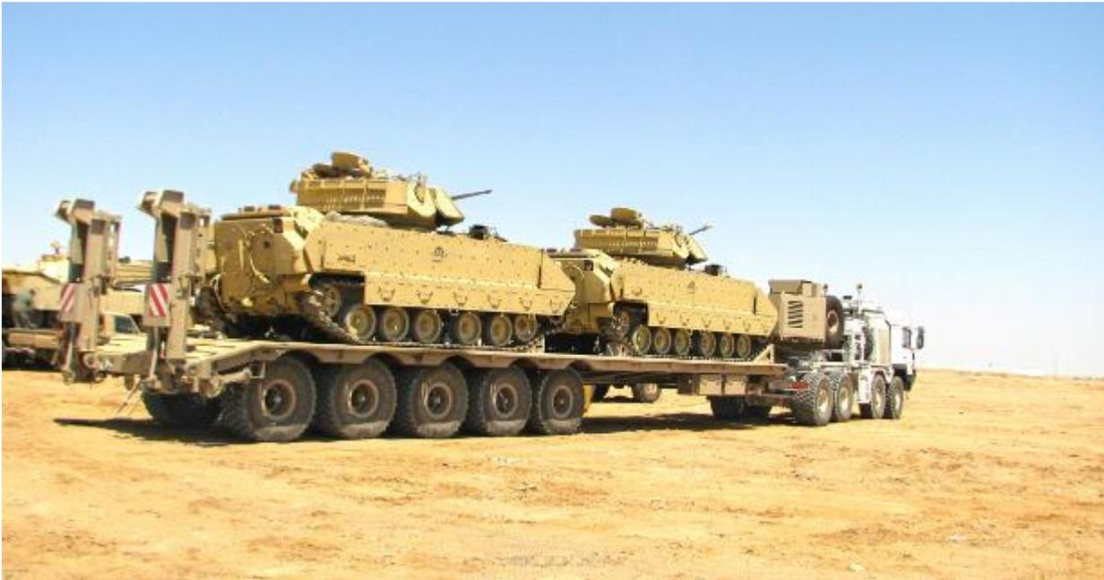
*Multiple loads: the PTL 70-90 can accommodate several vehicles at one time. A wide range of winches and loading aids is available for loading damaged vehicles.*
